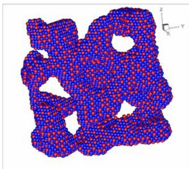
**Figure 5: Computer simulation of the Ni-Al leaching process to produce nanoporous sponge Ni (Al-red Ni-blue). [Courtesy: Swansea University]**
